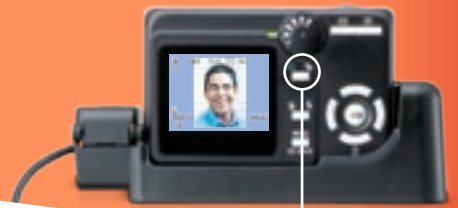
Press Print button for preview Press Print button again to transfer image data via USB to printer
